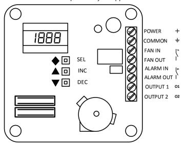
Senva recommends 14-24 AWG shielded twisted pair. For runs over 200 feet use a minimum of 22 AWG.
